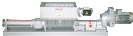
Pump type "T" with hopper and infeed screw with bridge breaker system driven by independent speed reducer. To pump dehydrated sludge from belt press - filter press.
