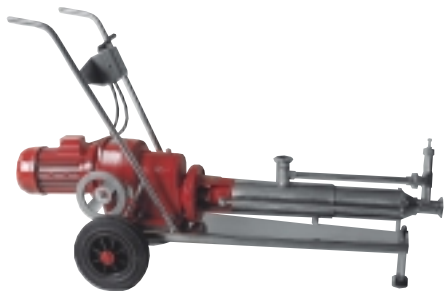
Pump type "US" in stainless steel execution with speed variator drive with automatic pressure safety valve and by-pass system. Application in the enological industry to pump wine-must etc.
