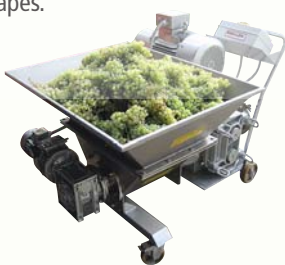
Rotary lobes pump type PL 4000 for pumping of whole grape
